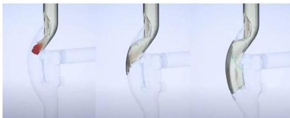
Fig. 4 - Simulation of swirl flow in the Sovent fitting [10]
