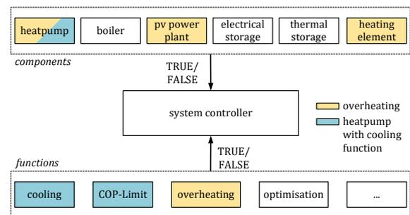
Fig. 3 – Possible assignments of the system controller
