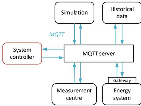
**Fig. 4** – Basic communication structure of the system
