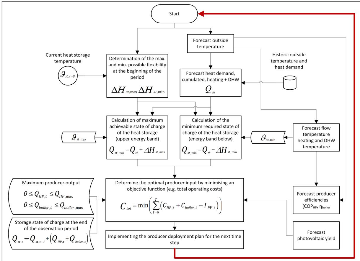
**Fig. 8** – Basic MPC algorithm
