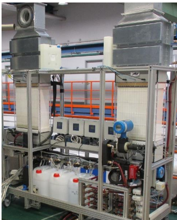
Fig. 6 – experimental setup of the 3-fluid closed-loop system for temperature and humidity recovery
