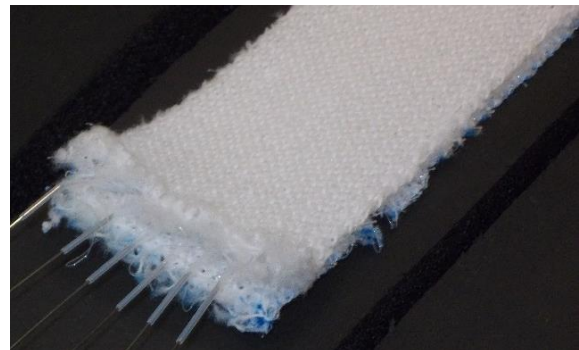
Fig. 3 – Flow-throughable spacer fabric (brine-side) with mechanically incorporated capillary tubes (waterside) for 3-fluid heat exchangers
