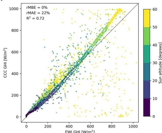
**Fig. 9** – Scatterplot showing the correlation between Global Horizontal Irradiance (GHI) values (in  $W/m^2$ ) recorded by a research grade pyranometer on a building on campus (EWI) and by the commercial pyranometer installed on the CCC roof.
