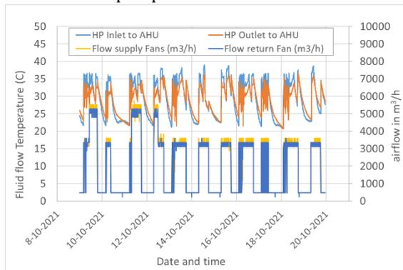
**Fig. 6** - Autumn measurement period (9 – 21 October). The fluid flow temperatures (around 35 °C) to and from the heat-pump to the heat exchanger (HP inlet and outlet to AHU) which heats up the air to the room and the air flows via the fans (m<sup>3</sup>/h) are presented.
