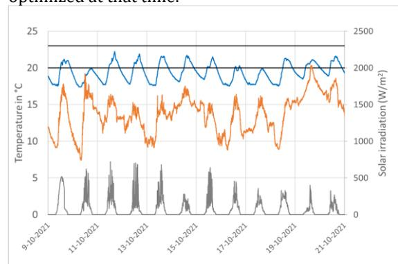
**Fig. 5** - Measurements 9 – 21 October 2021. The line at the top is the indoor temperature (blue) and, in the middle, the outdoor temperature (orange). The lower line is the solar irradiation ( $\text{W}/\text{m}^2$ ). The two black lines are the boundary conditions for occupied weekdays.
