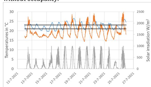
**Fig. 4** – Measurements 12 – 25 July 2021. The line at the top is the indoor temperature (blue) and in the middle, the outdoor temperature (orange). The lower line is the solar irradiation ( $\text{W}/\text{m}^2$ ). The two black lines are the boundary conditions for occupied weekdays.
