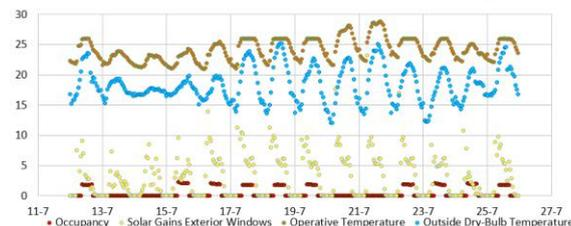
**Fig. 10** – DesignBuilder simulations for 12 – 25 July. The cooling set-point is 26/27 °C (adaptive range Category C). The operative temperature is shown at the top with the outdoor temperature below that line. The solar gains are low in summer: maximal circa 10 kW, due to usage of the blinds (circles at the underside). The dark line below those circles is the internal heat load. The left axis shows temperatures or kW's.
