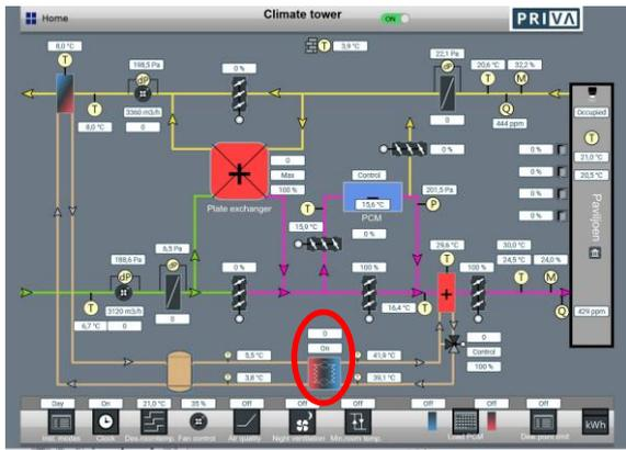
**Fig. 2** – Schematic overview of the climate tower and the sensors on the accompanying Priva website. The red box in the middle is the heat exchanger, the blue box the PCM-battery and at the bottom, circled, the air to air heat-pump can be seen.
