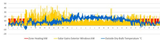
**Fig. 11** – DesignBuilder-simulations of the whole year. The set-point for cooling is 26/27 °C (adaptive range Category C). Red = heating load (kW), yellow solar load and blue outside temperature. The left axis shows the temperatures or kW's.
