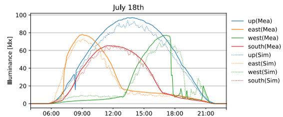
**Fig. 13** – Example of illuminance data recorded by the four roof sensors (solid lines) and corresponding results from the simulation (dotted lines), during a clear day (July 18<sup>th</sup>). The results for the west looking sensor are affected by nearby obstructing trees.
