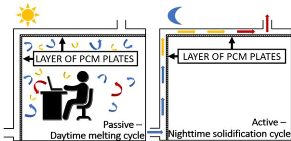
**Fig. 1** - Principle of the APS for cooling operation
