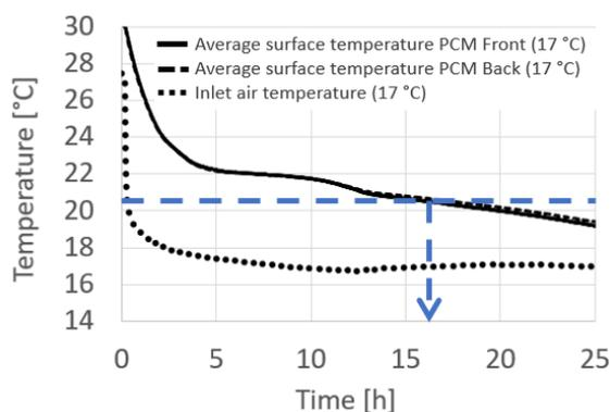
**Fig. 8** - The average PCM surface temperatures and inlet air temperatures obtained during the case solidified with average inlet air of 17 °C
