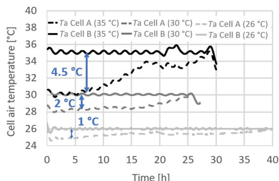
**Fig. 5** – Cell air temperatures obtained during the daytime melting cycle in cell A and cell B
