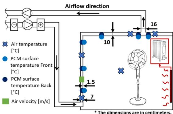
**Fig. 4** - Experimental features and measuring points
