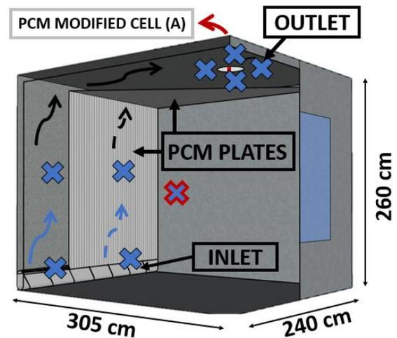
**Fig. 3** - Sketch with elements of the PCM modified cell
