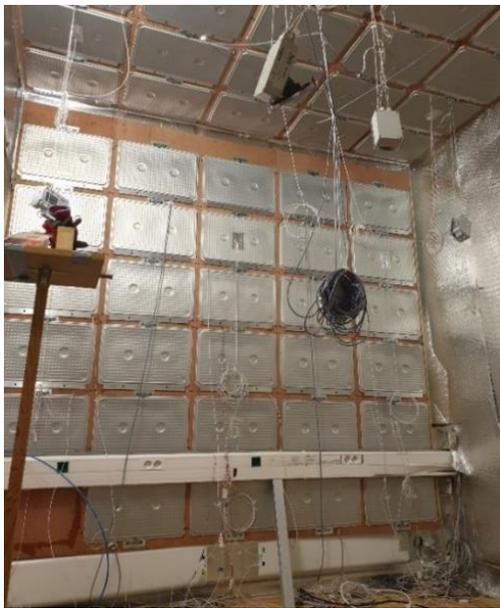
**Fig. 2** - Experimental facility (PCM modified cell)
