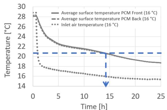
Fig. 7 - The average PCM surface temperatures and inlet air temperatures obtained during the case solidified with average inlet air of 16 °C
