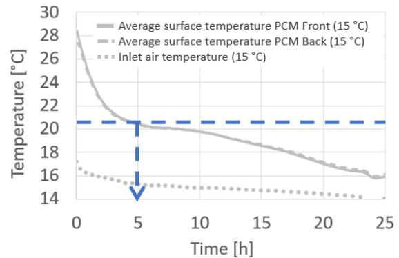
Fig. 6 – The average PCM surface temperatures and inlet air temperatures obtained during the case solidified with average inlet air of 15 °C
