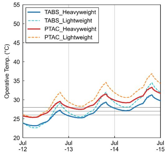
**Fig. 4** – Operative temperature of west office for the first 3 days of the heat wave (contemporary, with power outage).
