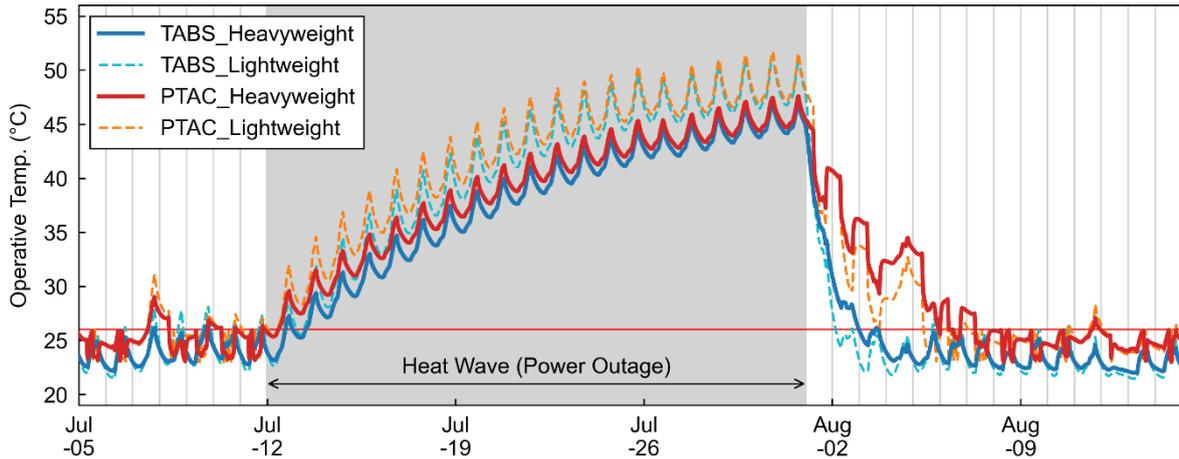
**Fig. 3** – Operative temperature of west office under contemporary heat wave conditions with power outage.
