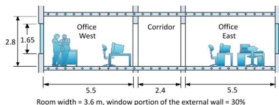
**Fig. 1** – Section view of building model (units: m) [10].
