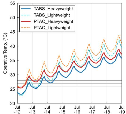
**Fig. 4** – Operative temperature of west office for the first 7 days of the heat wave (contemporary, with power outage).
