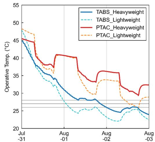
**Fig. 6** – Operative temperature of west office 3 days after the heat wave (contemporary, with power outage).
