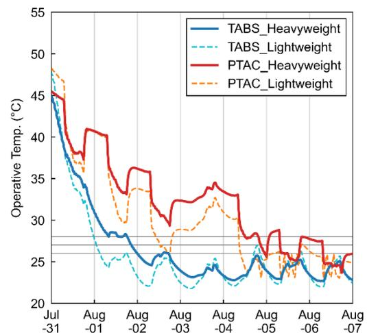
**Fig. 7** – Operative temperature of west office 7 days after the heat wave (contemporary, with power outage).
