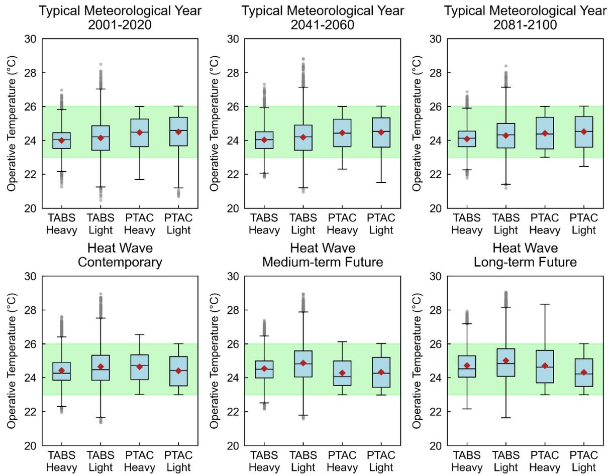
**Fig. 2** – Distribution of operative temperature in the west office during occupied hours.
