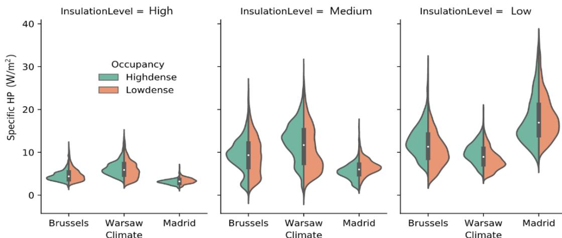
Fig. 3 Distribution of the specific maximum HP power in office cases related to different design parameters
