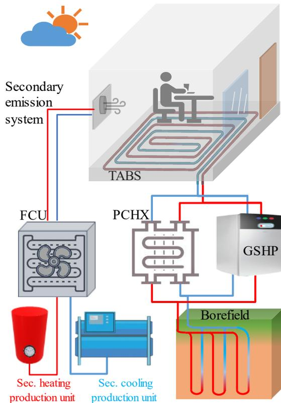
Fig. 1 key components of hybridGEOTABS [2]
