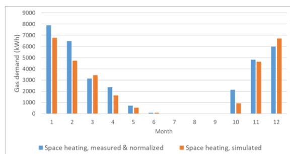
**Figure 2.** Measured and simulated space heating fuel use in the Spanish demo building.
