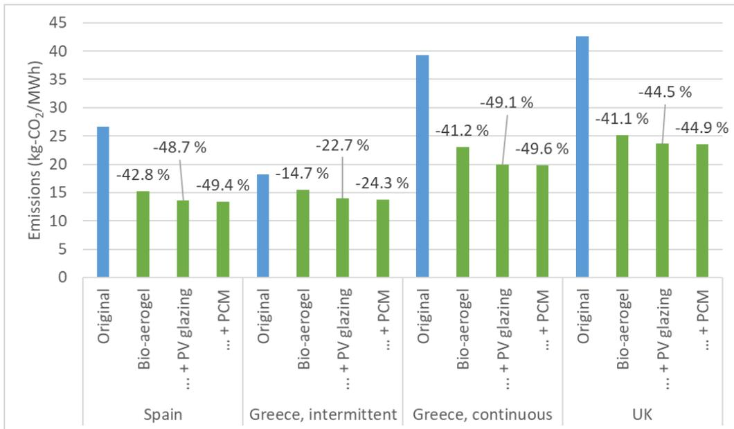
Figure 4. CO<sub>2</sub> emissions and relative reduction in each demo building before and after retrofitting.
