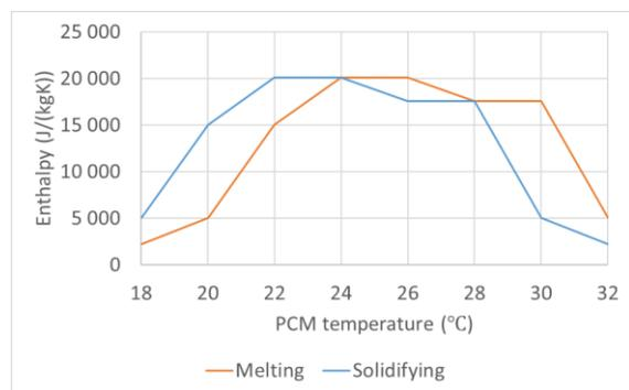
**Figure 3.** PCM enthalpies used in the simulation.
