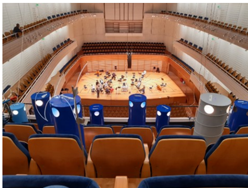
Fig. 5 – 3 rd Balcony of the concert hall with dummies and sampling points, view down to stage.
