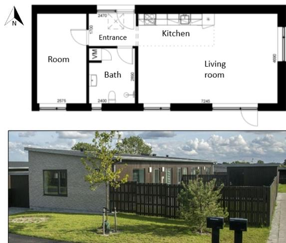
**Fig. 1** – Case building. Top: floorplan. Bottom: building illustration.
