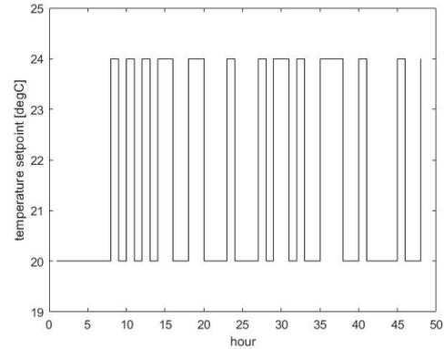
**Fig. 2** – Example of the PRBS signal (first 48 hours of the seventh order signal).
