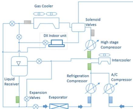
**Fig. 1** – Schematic of integrated CO2 unit
