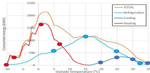
**Fig. 6** – Consumed energy distribution for non-integrated CO2 system
