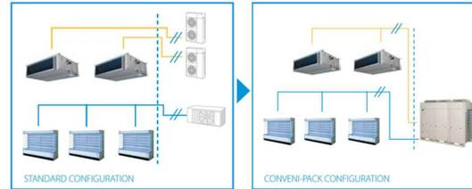
**Fig. 2** – Difference between non-integrated (left) and integrated (right) systems
