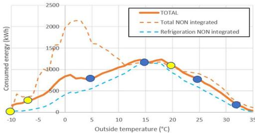
**Fig. 7** – Consumed energy distribution for integrated CO2 unit
