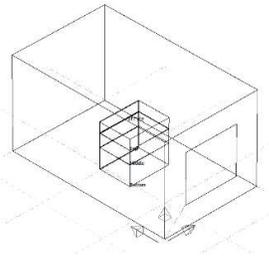
**Fig. 7** – One zone shoebox-model with “(Wo)Man in Cube”, window-to-wall ratio 30 %
