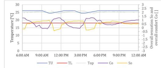
**Fig. 3** – One day simulation in summer with the adaptive building controller based on thermal sensation and comfort.
