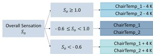
**Fig. 5** – Decision of the control logic of the adaptive building controller for the office chair with heating and cooling function, based on overall sensation  $S_o$ . ChairTemp\_1 represents the backrest, ChairTemp\_2 represents the seat.
