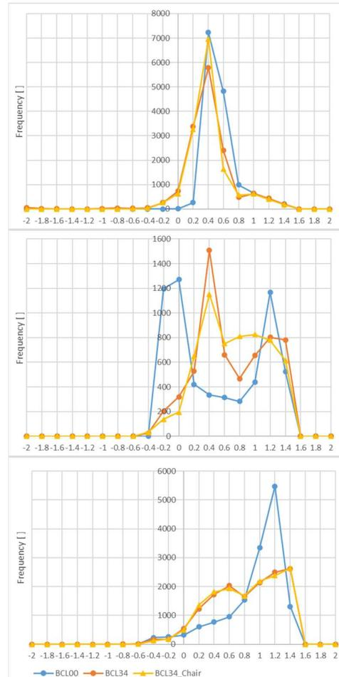
**Fig. 8** - Frequency of the comfort values for the period from a) 15<sup>th</sup> October to 15<sup>th</sup> March, b) 15<sup>th</sup> March to 15<sup>th</sup> May, c) 15<sup>th</sup> May to 15<sup>th</sup> October for the different controllers: Basic controller BCL00, adaptive controller BCL34, adaptive controller with office chair with heating and cooling function BCL34\_Chair
