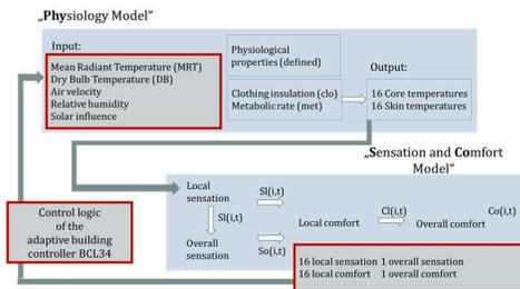
**Fig. 2** – Coupling of PhySCo within the virtual adaptive building controller BCL34 to maintain thermally comfortable conditions.
