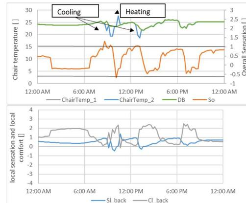
**Fig. 6** - One day simulation in August with the adaptive controller with chair. a) use of the cooling and heating function, based on overall sensation, b) local sensation  $S_i$  and local comfort  $C_i$  for the back
