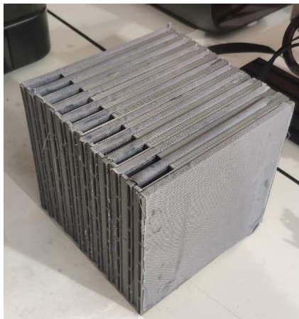
Fig. 5 – Heat and mass exchanger of the IEC system.
