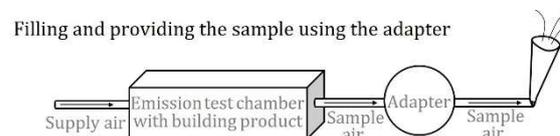
**Fig. 2** - Sample provision setup using adapter (single step).
