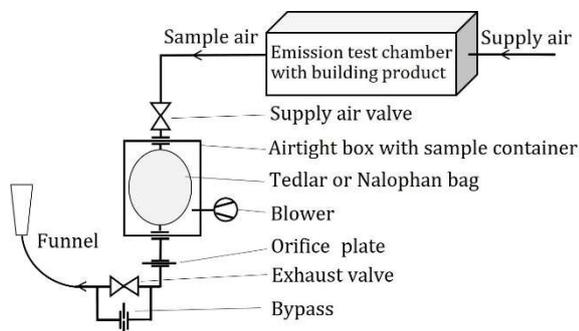
**Fig. 3** - Adapter setup and positioning.
