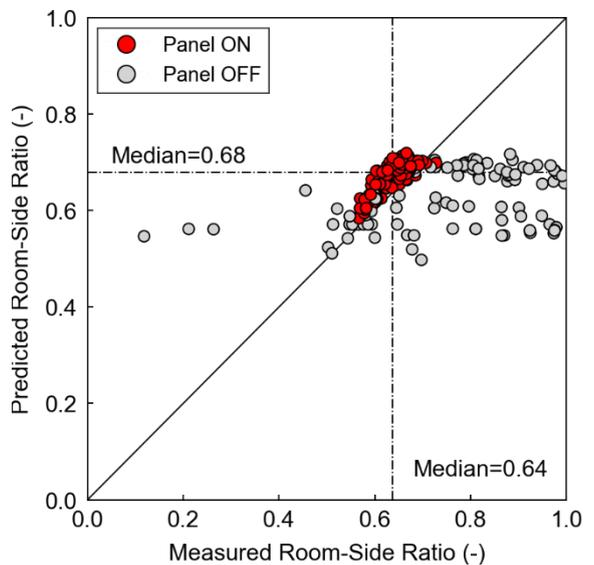
**Fig. 6** – Measured and Predicted Room-side heat flux ratio (all measurement period)
