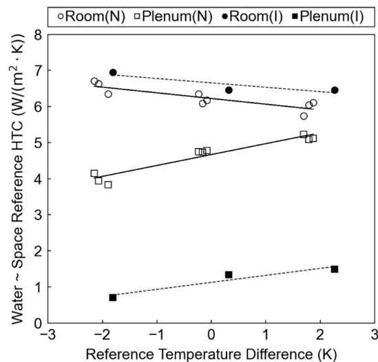
Fig. 4 – Empirical heat transfer coefficients (HTC: heat transfer coefficient, N: non-insulated panels, I: insulated panels)
