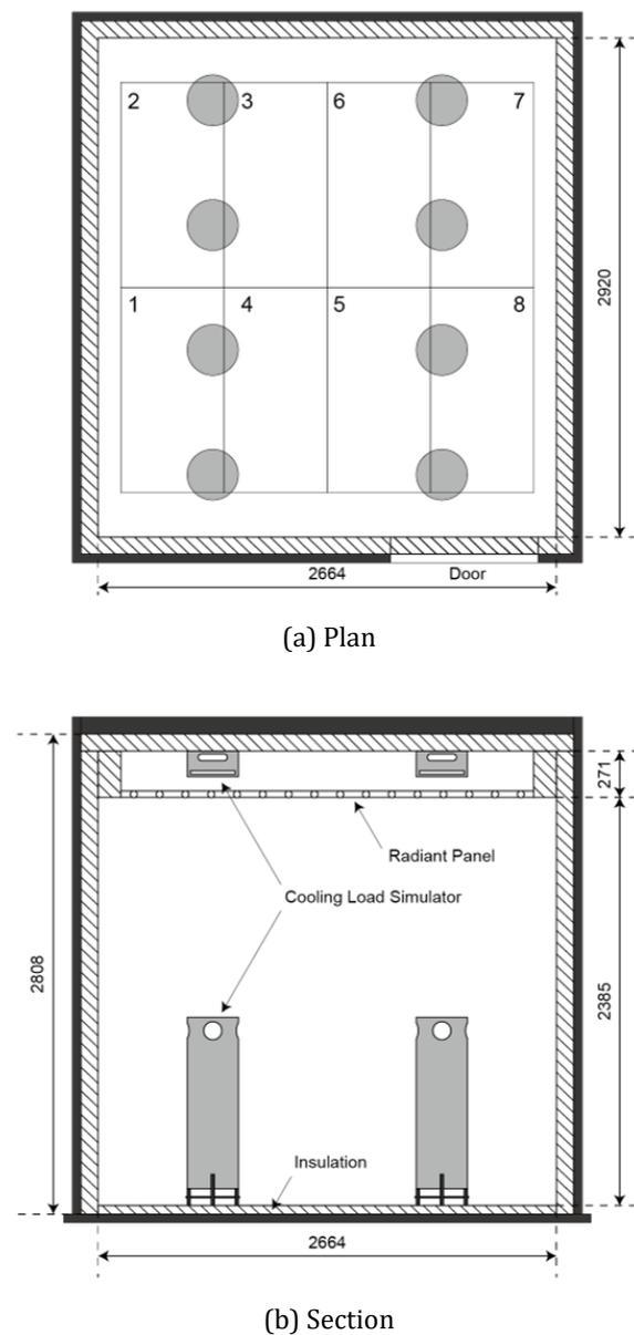
**Fig. 1** – Dimensions of the test chamber (units: mm).
