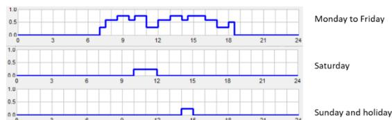
**Fig. 6** - The DHW consumption profile. The hours of the day are shown on the horizontal axis and the usage rate is shown on the vertical axis (0 = 0% usage rate, 1 = 100% usage rate).
