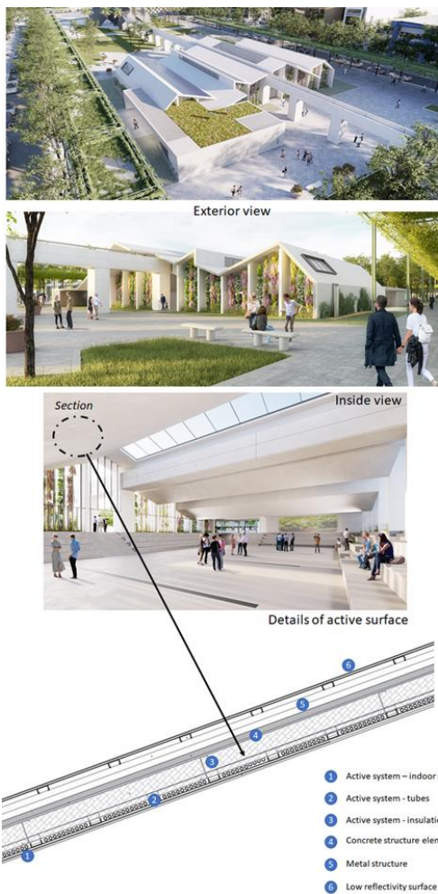
Fig. 8 - Design of climatic outdoor conditioning system by radiant surface in the souk.
